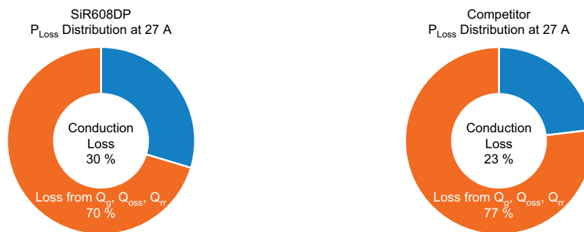
Fig. 4 - Power Loss Distribution for the SiR608DP and Competing Device at Output Load of 27 A
